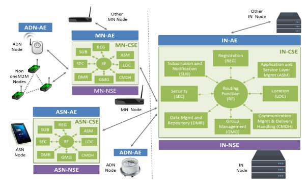
Figure 2 Eclipse OM2M functional architecture
